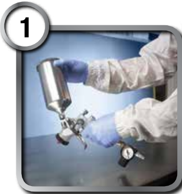
1 Remove existing cup from spray gun.
