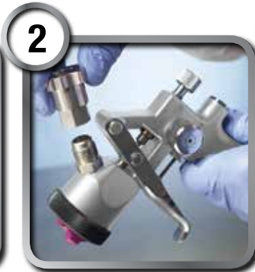
2 Thread correct adapter to spray gun.
