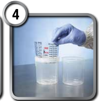
4 If not using a scale to measure, insert 3M™ PPS™ mix ratio film into cup before inserting liner in order to measure the paint according to paint manufacturer's guidelines.
