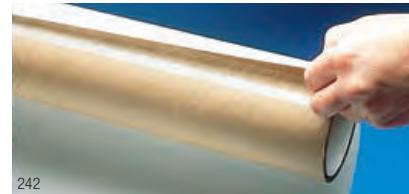
242 High tack side of 3M™ Removable/Repositionable Tape 9415 “permanently” adheres to cores for winding up paper or film. Low tack side releases the paper or film when unwinding.
