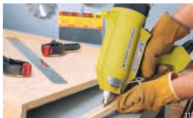
Adhesive bead applies neatly to countertop edging to eliminate nails and the extra work of putty and sanding.
