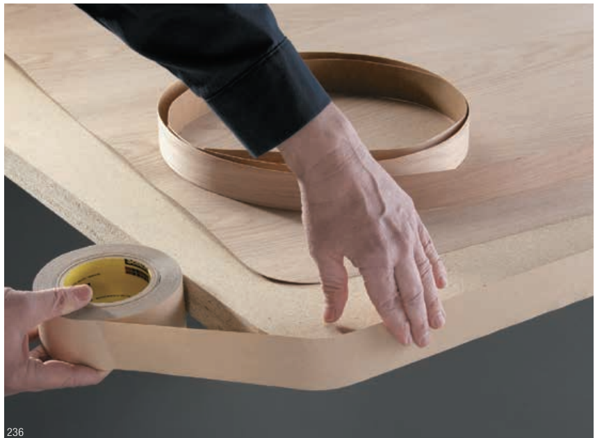
236 Simply roll on a strip or band of 3M™ Double Coated Tape 9832 for quick edge banding with no special equipment. Pressure sensitive adhesive tape grabs with immediate handling strength for improved productivity.
