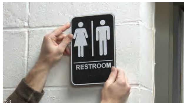
3M™ Double Coated Urethane Foam Tapes bond plastic signs to painted cinder block. The foam fills gaps between irregular surfaces. Various foam thicknesses are available for surface conformance based on the degree of roughness.
