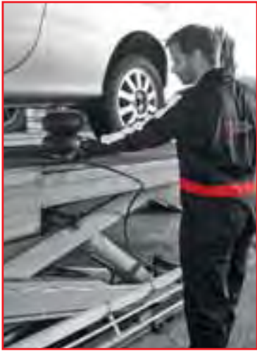
Balloon jacks can be used on column lifts. Ideal for tire changing applications and bodyshops
