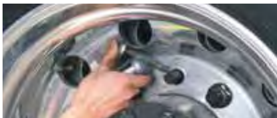
STEP 5 Place two drops of oil near the end of the stud.
