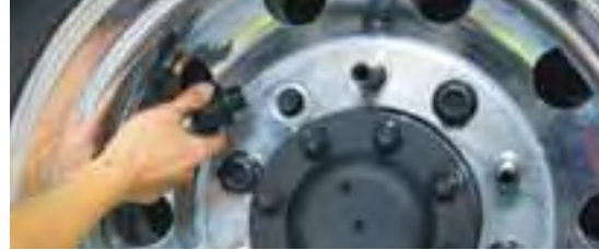
STEP 7 Install the nuts by hand.
