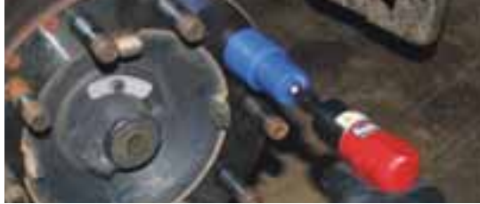
STEP 2 Clean the drum and studs. Inspect for fatigue with thread gauge.
