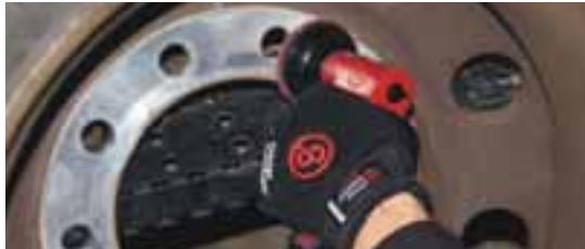
STEP 3 Thoroughly clean both sides of each wheel with the CP7202D sander and an appropriate abrasive. Inspect all surfaces for cracks and unusual wear.
