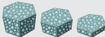
The three-dimensional structures of 3M™ Trizact™ Abrasives contain multiple layers of mineral. As these structures wear, fresh, sharp mineral is constantly exposed to the workpiece, resulting in faster, more consistent cutting throughout the life of the belt.
