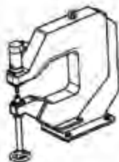
Assembly for riveting fastened to fixed frames examples
