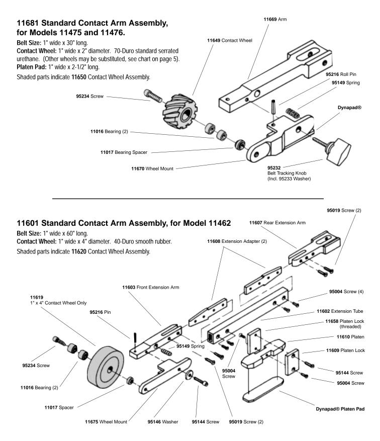
The **11462** Dynabelter<sup>®</sup> Finisher normally uses 1" wide x 60" long abrasive belts. The **11602** Extension Tube can be modified to accommodate various belt lengths.
