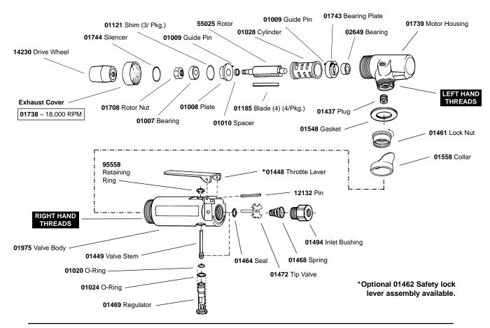
Heavy-Duty Air Motor 07100 — Powers Model 11476 Dynabelter® (Includes 11518 Drive Wheel)
