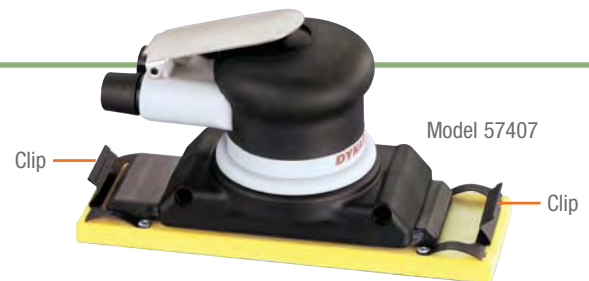
Dynaline achieves in-line scratch pattern on stainless steel by powering non-woven nylon abrasives on long nap hook-face pad.
