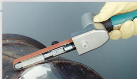
DYNAFILE® II Grinding head pivots 360°; 7° offset handle. Easily converts to Die Grinder and Drill.
