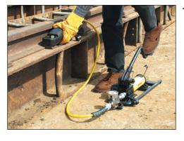
Easily removing rusty nuts during railroad construction is just one of many application examples for the Enerpac Nut Cutters.
