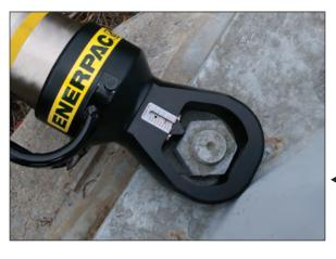
◀ Heavily corroded and weathered nuts are quickly split and removed using an NS-Series Nut Splitter.
