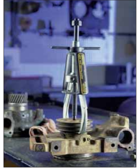
▲ EP-204 2-jaw puller positioned to pull a water pump drive pulley.
