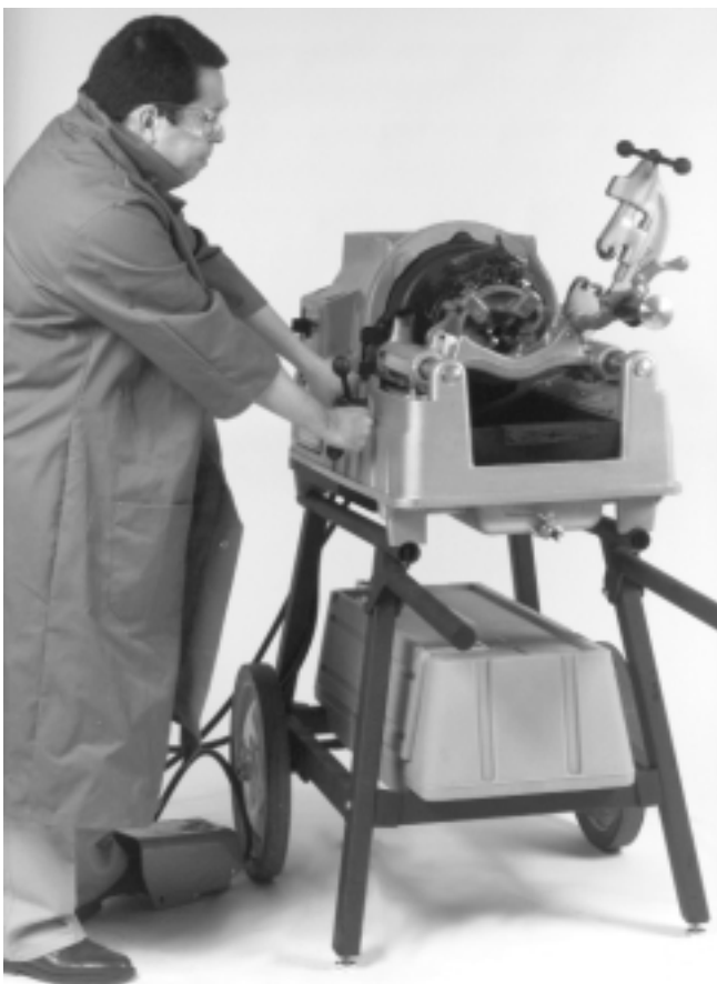
Figure 8 – Threading With 535 Automatic Threading Machine
