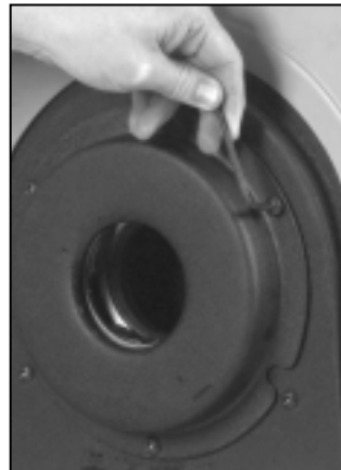
Figure 18A – Removing Rear Chuck Cover
