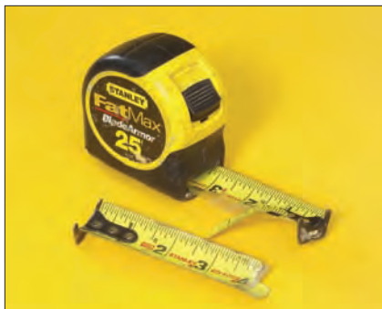
Torn or Damaged Blade
