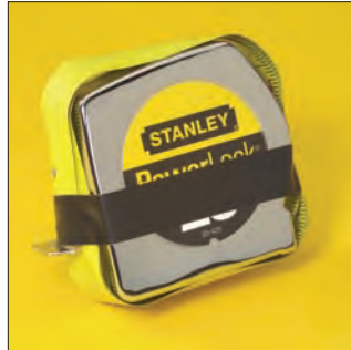
Broken Spring; Blade Will Not Retract
