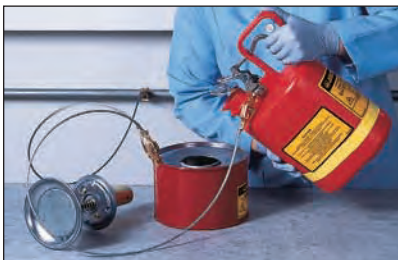
Grounding with antistatic wires
