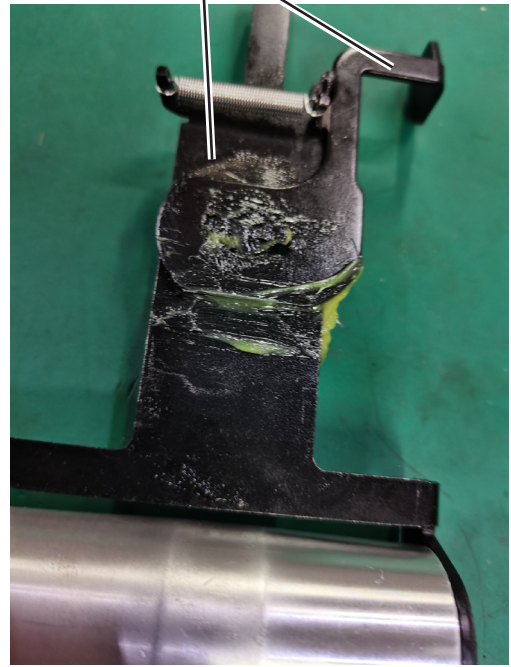
Apply 0.2g of Type "J" grease (49-08-4175) to tension bracket and tension lever
