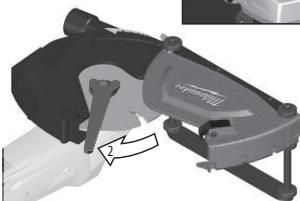
10. Close the wheel cover and ensure the shroud button is snapped in place.
