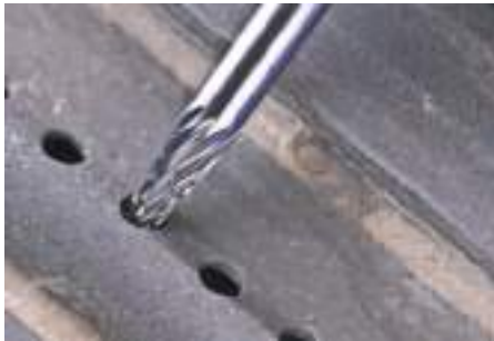
Conical burr with pointed end. PFERD specification number SKM
