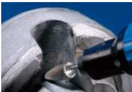
Tree-shaped bur with radius end.
