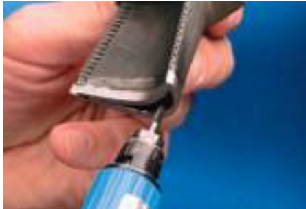
Cylindrical bur with end cut.
