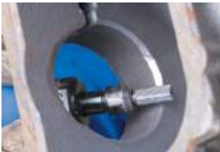
Cylindrical bur with end cut.
