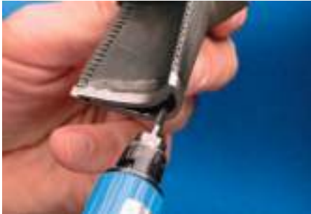
Cylindrical bur with end cut.
