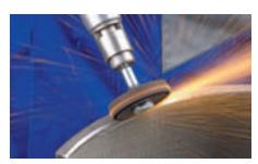
Accessory for mounting snagging wheels on straight grinders.
