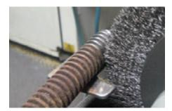
Medium face brushes are designed for medium to heavy duty use either individually or gang mounted. As with all PFERD crimped wire wheel brushes, the metal components and adapters are designed for a flush fit when gang-mounted. This design ensures a consistent, seamless surface finish. Also recommended for bench/pedestal grinders.
