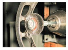
These small diameter wire wheel brushes are designed for use in restricted or hard-to-reach areas. They are excellent brushes for deburring, blending, and cleaning of surfaces and cavities.
