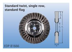
Standard twist knot wheel brushes feature knots that are twisted approximately 75% of the length of the trim. The loosely-twisted knots cover a larger surface area and are ideal for heavy-duty cleaning and surface conditioning. For weld cleaning, weld spatter removal, scale removal, cleaning, deburring, and flash removal.
