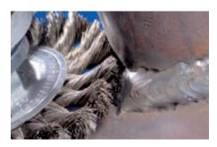
Narrow face allows better control of surface contact area. Full cable twist is ideal for the tough brushing applications where surface finish is a low priority.
