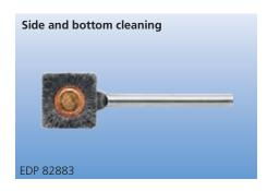
Side and bottom brushes are ideal for cleaning the side and bottom of blind holes. The brush face can also be turned 45 degrees to clean snap ring grooves and other recessed features. Mount in drill press or portable tool.
