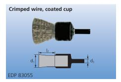
General purpose for working hard-to-reach places. For use on portable air and electric tools. Used for rubber and plastic flash removal, paint and rust removal, die, mold and tool polishing. Coated cup version features elastomer sleeve to protect against contamination.
