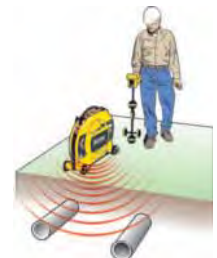
Induce a signal to locate utilities.
