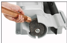
The optional Debur Disk is used to grind the O.D. edge to help with tight fittings
