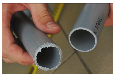
Cut with a hacksaw (left) versus the P-TEC 3240 (right).
