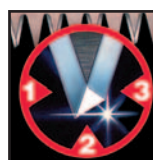
SHARPTOOTH™ TECHNOLOGY UTILIZES THREE CUTTING SURFACES.
