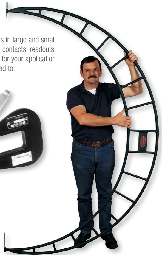
Starrett can manufacture extra large micrometers, like this special 724 Micrometer of tubing type construction, range 72-78" (1800-1950mm), with interchangeable anvils.
