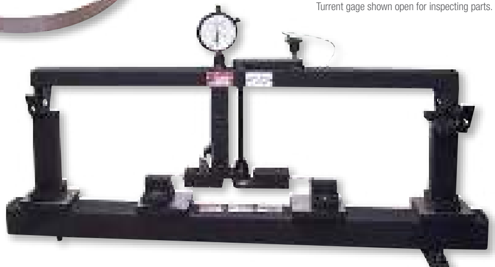
Turrent gage shown open for inspecting parts.
