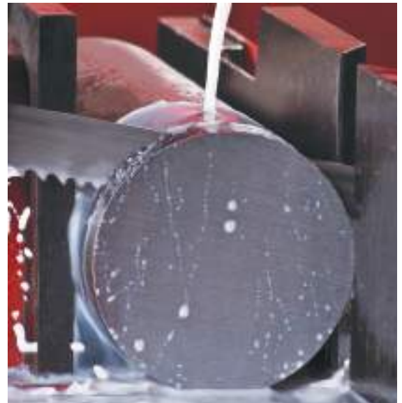
After break-in when the blade has fully entered the work-piece, increase the feed rate over a series of cuts until the recommended cutting rate is achieved.
