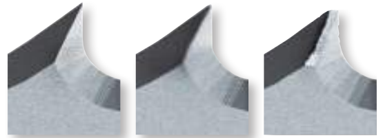
Tooth correctly broken in
