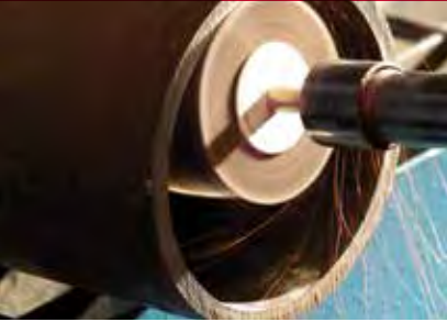
Removing burrs from the inside diameter (ID) of a cut tube.
