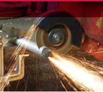
Cutting a piece of bar stock with an UltraCut wheel.
