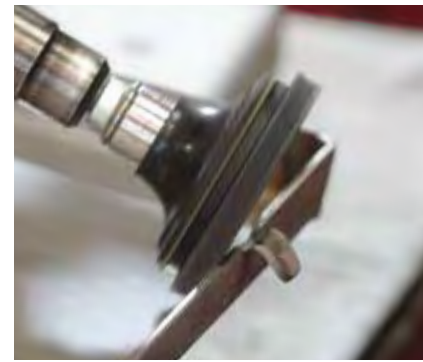
Edge chamfering a fabricated stainless component.
