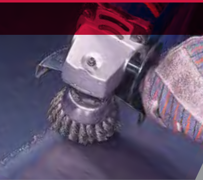
Removing slag from a flame-cut steel plate.
