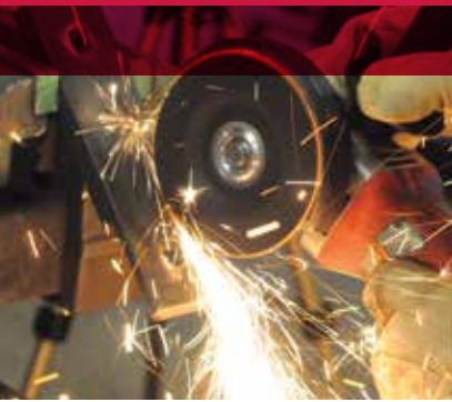
Cutting a v-groove in bar stock with a Tiger Cutting Wheel.
