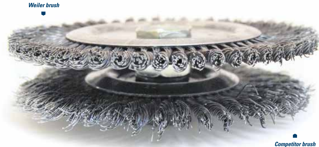
Stringer Bead Wheel Brushes tested for 30 minutes at 6,000 RPM against a piece of steel diamond plate using 12 lbs. of pressure.
