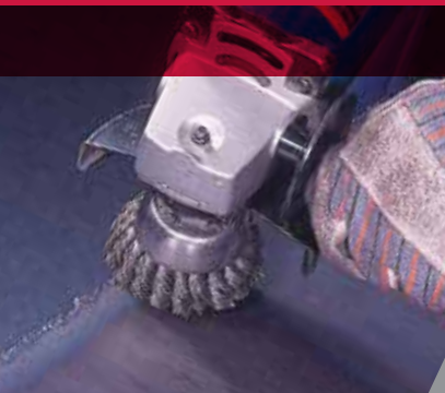
Removing slag from a flame-cut steel plate.
