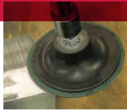
Blending welds and saw marks on a mounting bracket.
