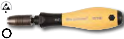
38701 ESD Safe Quick Release 1/4" Bit Holder, With Wiha-SoftFinish® Cushion Grip Handle, IEC 61340-5-1, DIN 3126, ISO 1173 Stainless steel with retaining ring bit holder. Dissipative SoftFinish® cushion grip handle, multi-component, ESD Safe surface resistance 10 6 - 10 9 Ohm.
